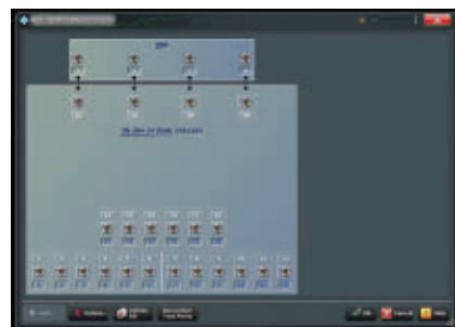
▲ Fig. 2 The connected switch matrix is shown in the VNA firmware menu. This example shows a 4 \times 18 switch matrix.
