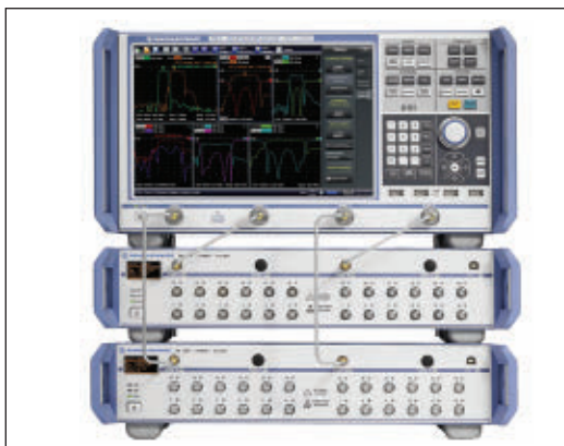
▲ Fig. 1 A test solution with 48 ports consisting of one R&S ZNB8 and two R&S ZN-Z84 switch matrices.
