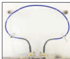
Flex Test™ setup shows triple strain relief, effective through 20,000 flex cycles for all models.
