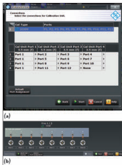
▲ Fig. 3 Overview of the calibration of twelve ports using a four-port calibration unit (a) and the first calibration step using an eight-port calibration unit (b) four calibration steps are necessary.
